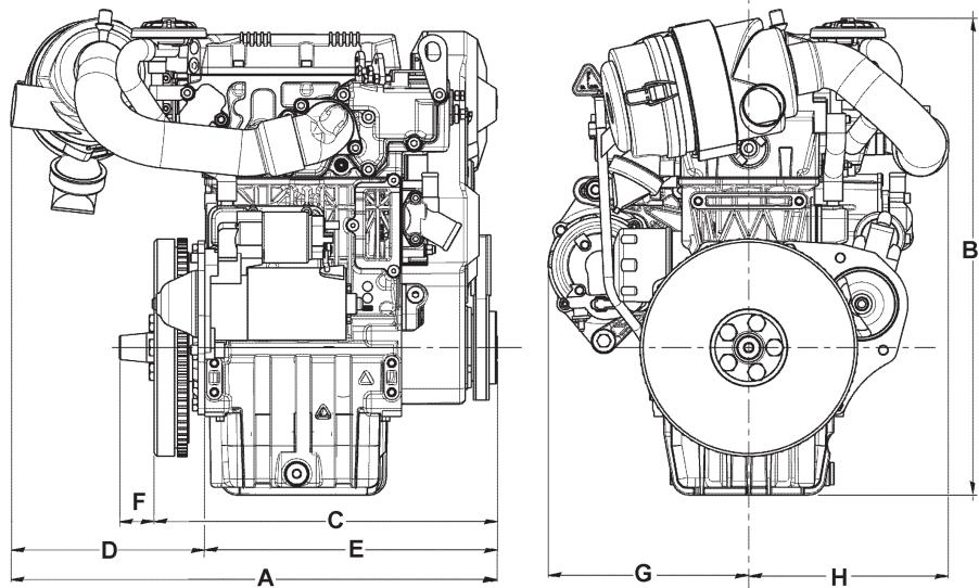
DIMENSIONI mm - MESURES mm - DIMENSION mm - EINBAUMAßE mm - DIMENSIONE mm - DIMENÇÕES (mm)
