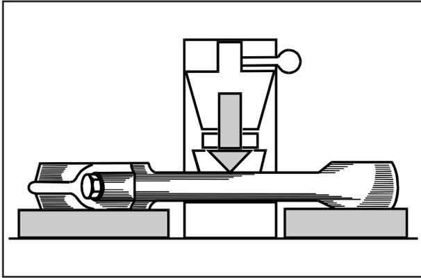
The operation is carried out by applying a calibrated pressure to the convex side in the middle of the connecting rod stem set on surface plates (fig. 20).
