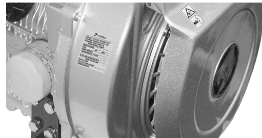
Data plate for EPA Standards applied to the air intake cowling.
