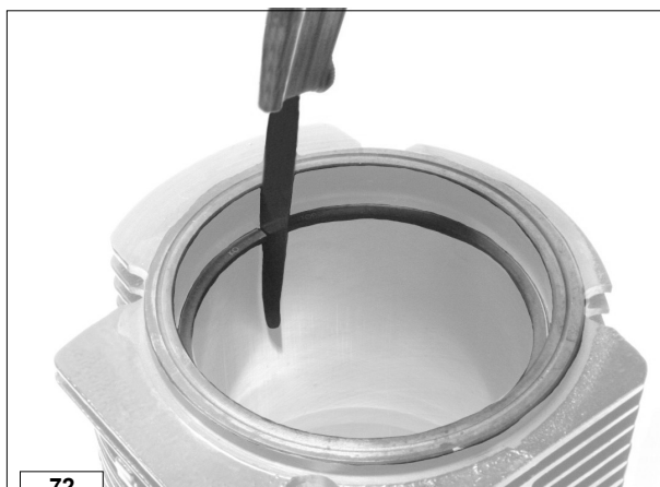
Piston rings, distance between the tips (mm)
