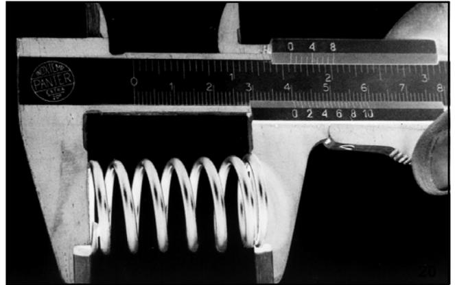
The permissible tolerance for load and length is: + or - 5%. If these values are not achieved, replace the spring (fig.20).
