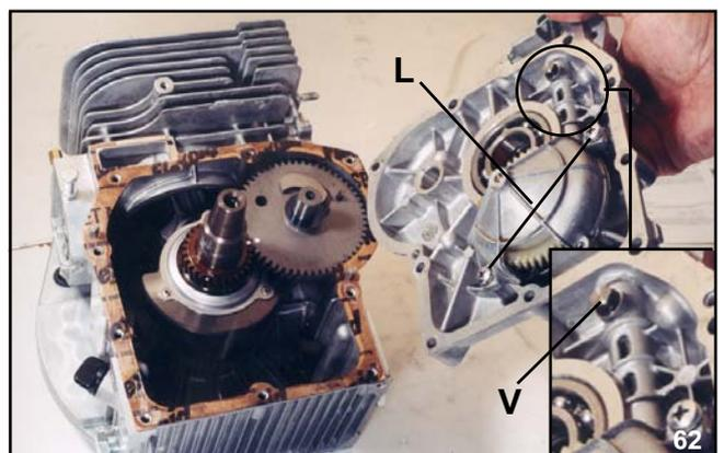
**N.B.:** care should be taken when mating the governor gear with the crankshaft gear. Do not force the cover if the mating has not been carried out correctly, as this action may result in serious damage to the governor gear.
