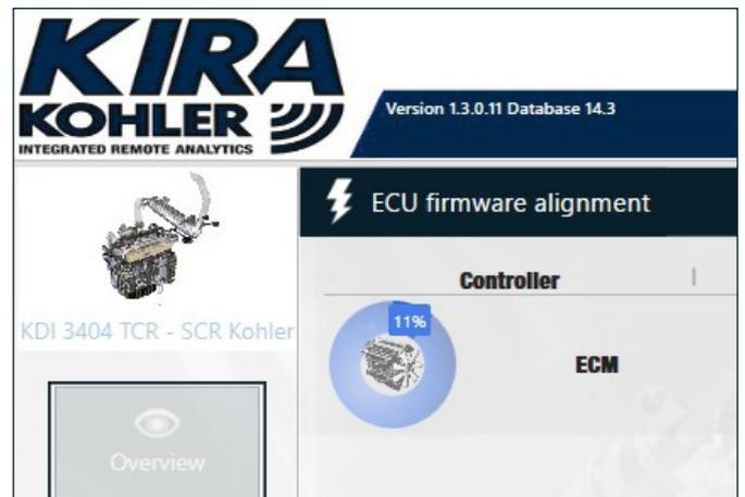
Once the download is completed, the tool will perform a flashing of the control unit. The actions that the user must perform to complete the operation are displayed in this process as well.
