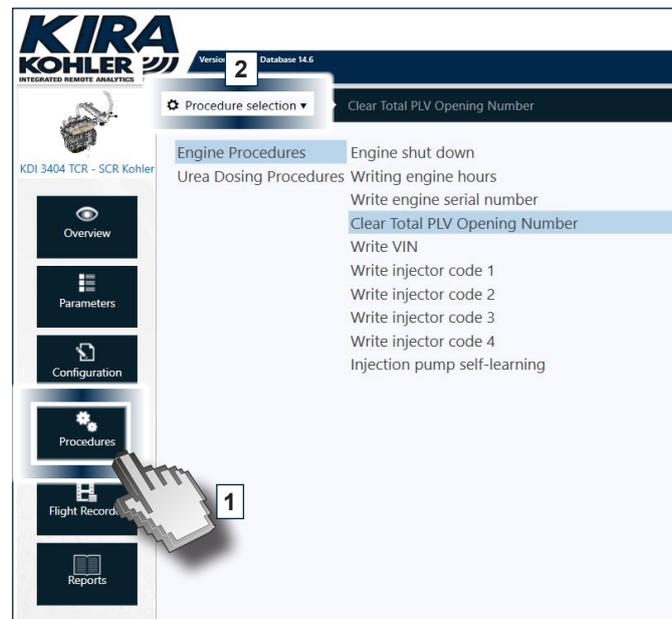
An example of a guided procedure is provided below. Click on "Engine procedures" and "Engine shut down".
