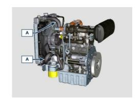
1. Check the integrity of the pipes and hoses A.
